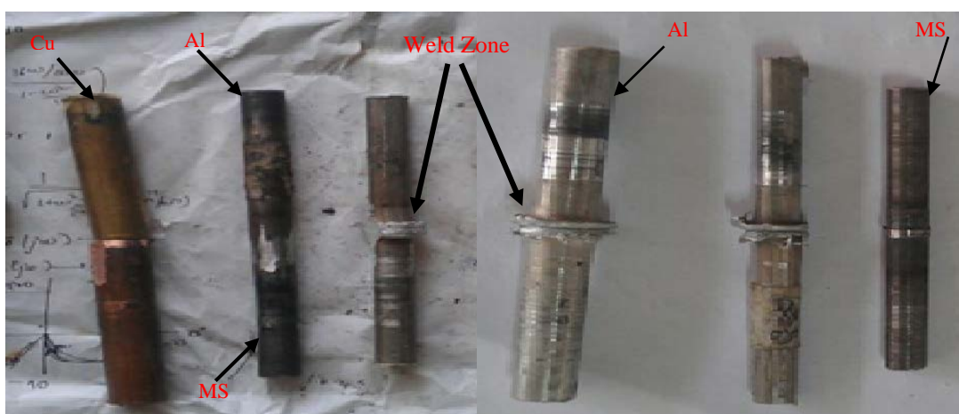
Fig.5. Rotary Friction Welded specimen for similar and dissimilar
